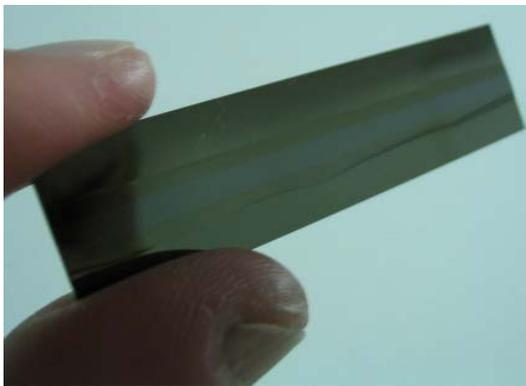
Waveguide on Silicon Substrate
