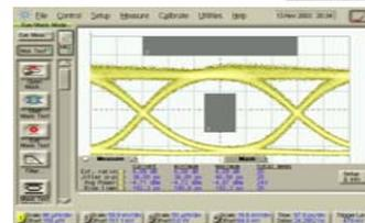
Eye diagram of array transmitter
