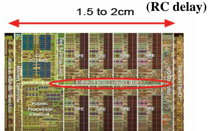
Cell processor (IBM/Toshiba/Sony)
